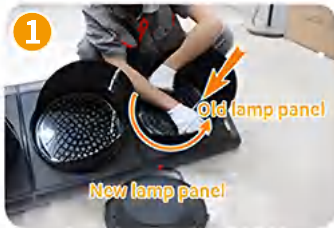
Remove the original lamp panel
