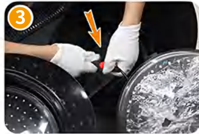
Unscrew the cable and unplug it
